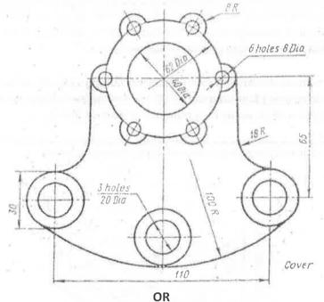
Q.1(B) Draw the below figure using Auto CAD commands
