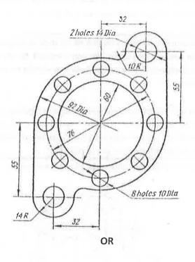
Q.1(B) Draw the below figure using Auto CAD commands
