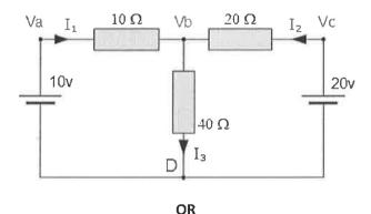
Q.2(B) Find the current through each resistor in the circuit shown below using Mesh analysis
